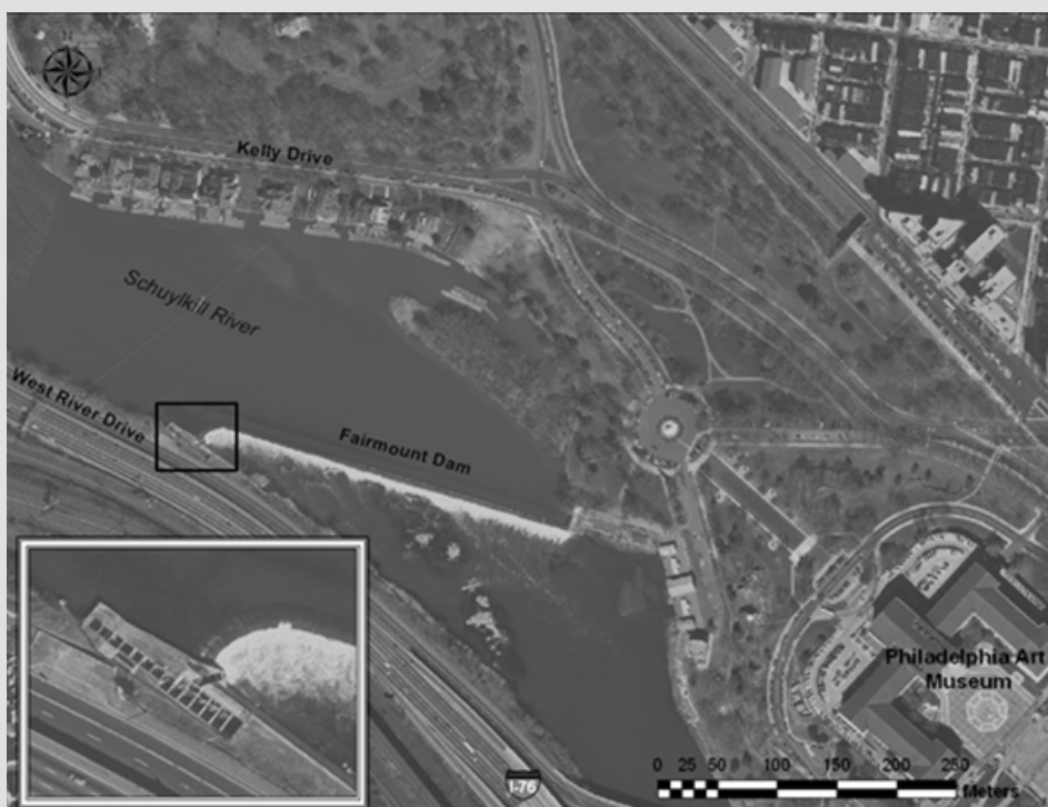
Figure 6.8.9.1 Aerial view of Fairmount Dam and vertical slot fishway (left insert) located on the west bank of the Schuylkill River at river km 13.6, Philadelphia, Pennsylvania. Courtesy: Perillo and Butler (2009).
