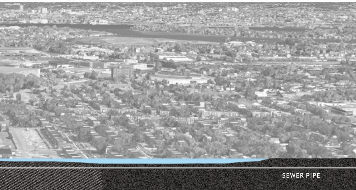
Image 2: The Delaware and Cooper are both tidal rivers directly connected to the ocean. As sea level and storm surges have risen over the last 100 years, the ends of the sewer pipes are underwater more of the time, and unable to release runoff to the rivers until water levels drop. Source
