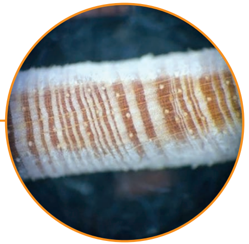
A sanded tree core image enlarged under microscope. Rings tell researchers a tree's age and the conditions under which the tree grew from year to year. When conditions are good, trees grow thick rings. Rings are thinner when growing conditions are less optimal.
